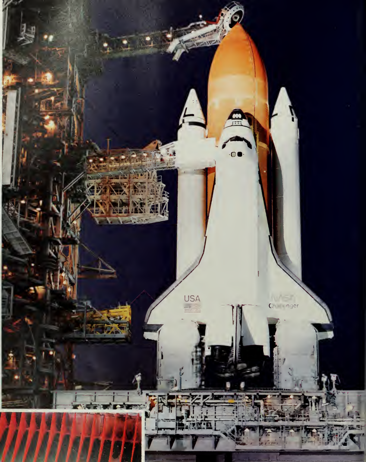
Above, Shuttle 51-L on Kennedy Space Center Pad 39B in the early morning of launch day. Temperatures were well below freezing, as indicated by the lower left photo, which shows thick ice in a water trough despite use of an anti-freeze solution.
